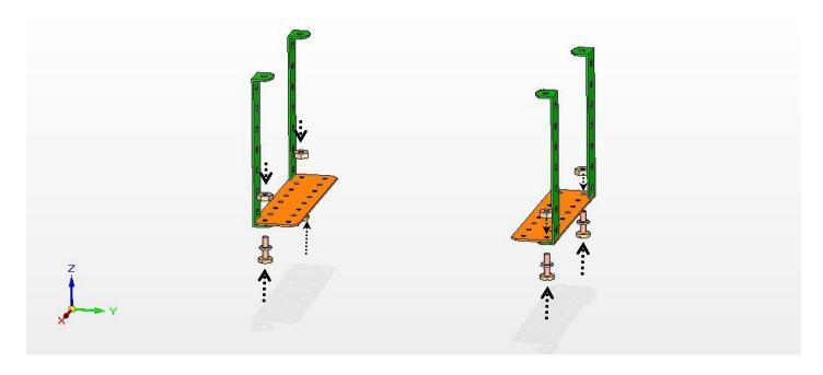
Step 3: Take DB12 and connect to the top of the UC7\*1\*1 connectors
