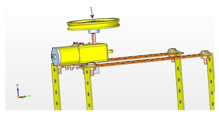
**Note:** Screw it with the help of screw to tighten the pulley to motor axle.
