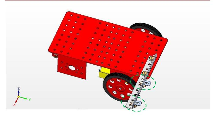
**Step 5:** Fix the Servo motor to the UL1\*1 connector with the help of two M3S screws as show below.
