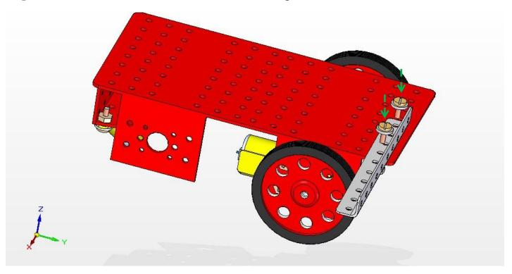
**Step 4:** Connect two UL1\*1 to the LS10 beam with the help of M3S Screws as shown in the figure.
