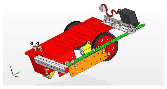
Note: See the LS10 strip should not touch the FB16 beam (green component shown in the image).
